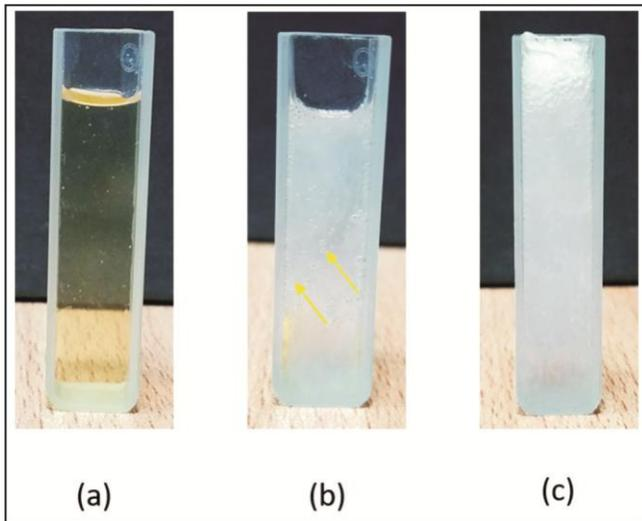
**Fig. 3:** Sequence of pictures illustrating physical changes occurred at 37°C. (a) Clear solution mixture before gelation. (b) Gelation started at 37°C. (c) Gelation completed at 37°C. Yellow arrows are indicating effervescence of CO<sub>2</sub>.
