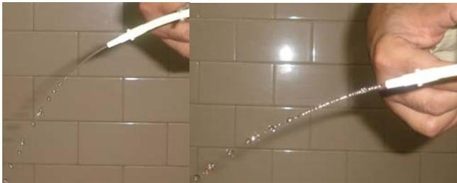
**Fig. 6.** Flow less without air pump(Left) and increasing with air pump on (Right).
